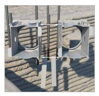
In order to implement the standardised centre distance of 71 mm for combinations, the contact area must be cut off at the rear markings.
