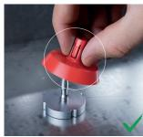
... that the latches remain free so that they can release the magnet.
