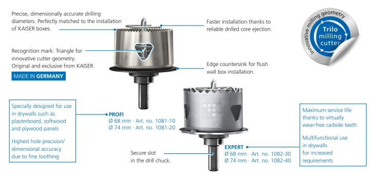
The innovative Trilo geometry of the cutter head ensures for an optimised cutting performance and an improved operating life. In combination with the new centring drill, reliable ejection of the drilled core is possible and facilitates fast work.
