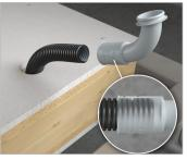
The protruding electrical installation conduit is inserted into the conduit holder of the 90° bend up to the depth stop and locked together.
