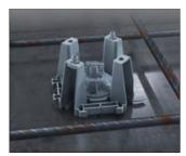
By putting on the integrated closing cap, the interface of the system magnet is protected from concrete on the rear side.
