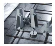
The fixing of extension element 48.5 mm (Art. No. 1261-02) for use in automated production lines is carried out via...
