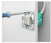
Secure the installation accessory with the device screws.
