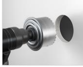
Create installation opening Ø 68 mm with KAISER cutter (e.g. MULTI 2000 HM, Art.-No. 1083-70).
